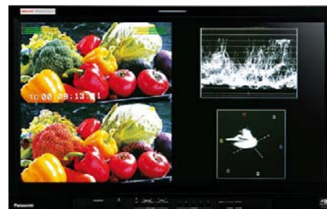
Sample display of the input source image (upper left), Focus-in-Red (upper left), WFM (upper right) and VSC (lower right) (All images are simulated.)
