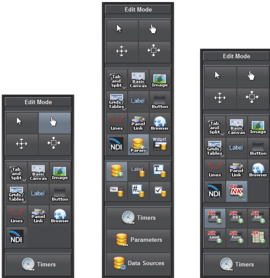
Figure 5.5 - Three Versions of the Edit Mode Toolbar (without associated data source, with associated data source, and including router control buttons)
