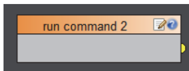
Figure 6.17 - A Logic Block with an Output but no Top or Bottom Connectors
