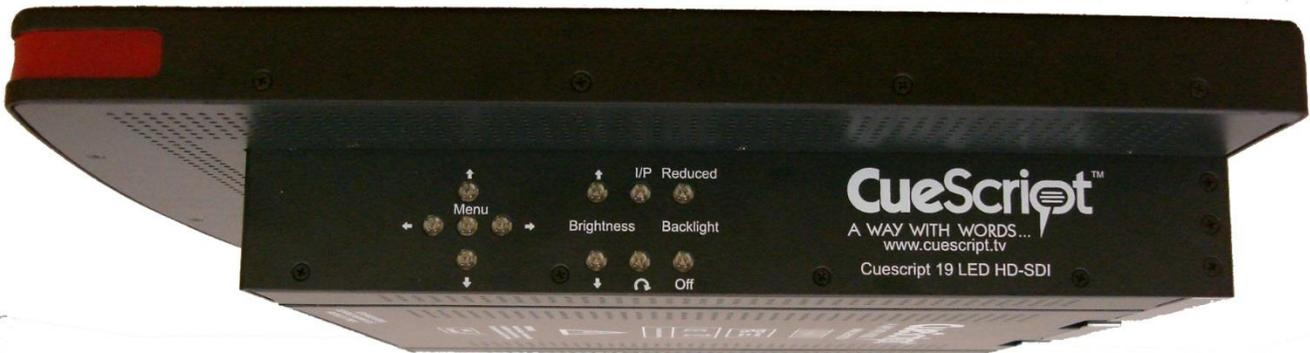
There are 11 buttons on the right side of the prompter. All of these buttons are illuminated and nine of them increase brightness when touched. After a short period of time when no buttons have been pushed, they will revert to their low brightness level. The two backlight inactivity control buttons have fixed brightness levels.
