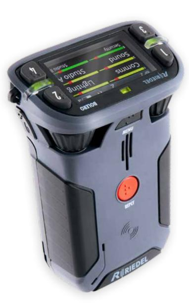
Bolero runs over a standards-based AES67 IP network with decentralized antennas connected to AES67 switches and to Artist frames equipped with AES67 client cards, providing a fully integrated point-to-point roaming intercom ecosystem. The more decentralized antennas added, the more robust the network becomes.
