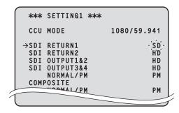
Once the setting value has been confirmed, the flashing stops, and the cursor can be moved from one menu to another.
