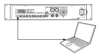
Set an IP address for the computer within the private address range while ensuring that it is different from the address of the unit. Set the subnet mask to the same address as the unit.
