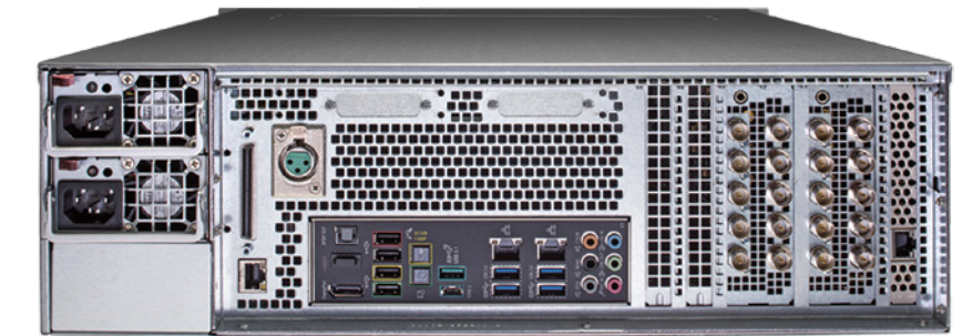
Mira Production Server Chassis – Rear Panel
